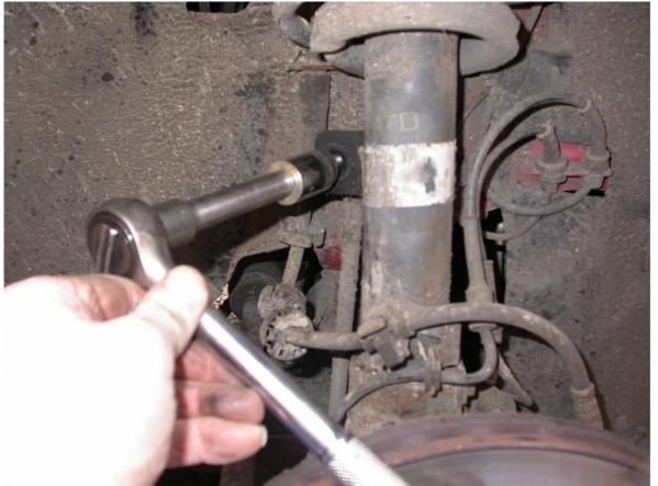
4. Carefully apply some WD40 and remove the top locking nut (18mm) on the anti-roll bar link (where it attaches to the strut). It will not be possible to remove the link at the moment – see operation 8.
