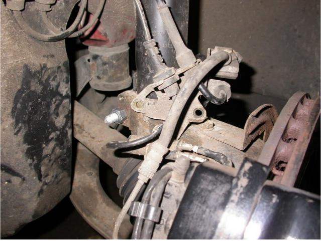
5. Remove the 2 (10mm) bolts holding the clips for the brake hoes and pad wear sensors – this is just to help improve access and allow you to remove/refit the parts
